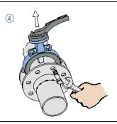
Unscrew the bolts and nuts and get the valve out
