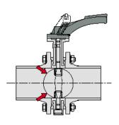
Check again the opening and closing of the valves to make sure that it's operating well, especially that the disc operation to the fully open position will not be obstructed.
