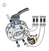
As illustrated above, insert 4 bolts and screw in the nuts slightly.
