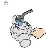
Position the valve against the mating flanges and tighten 4 bolts and nuts gradually. (Take care not to over-tighten the nuts and bolts.)
