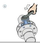
After welding seams cooled down, slide in the butterfly valve. Make sure there is enough space for the valve and the disc is slightly open.
