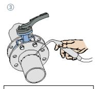
Fix the flange onto the pipeline by means of spot welding
