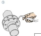
Weld the flange with the pipe securely
