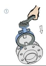
Put the butterfly valve between the two mating flanges to be installed on the pipeline.
