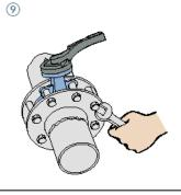
Tighten all the bolts and nuts evenly. (When do the tightening, do it with the opposite two bolts and nuts alternatively)
